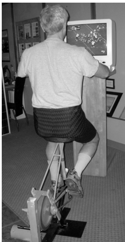
A fit person can pedal at the rate of 200 watts, enough to power a 19" TV, as long as he keeps pedaling vigorously.
